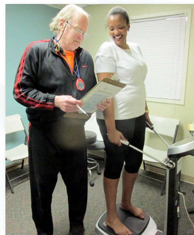
InBody®: BIA Bioelectrical Analysis, including a Body Composition Analysis (weight, lean body mass and body fat mass), Body Water Balance (intracellular water, extracellular water, and total body water), Obesity Diagnosis (BMI, or body mass index, and percentage of body fat), and Segmental Lean Development
